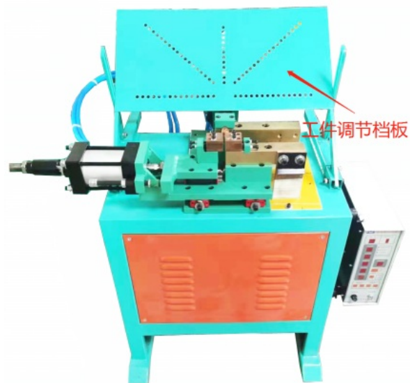
4. The special workpiece adjusting baffle can support the workpiece and adjust the welding angle of the workpiece for large workpieces, which is very useful.
